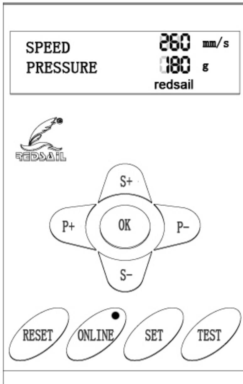
The main screen of the cutter allows you to set the main settings of the cutter including the cutting speed and cutting force options. It also allows you to cut a test pattern or check the amount of force that is currently set.
