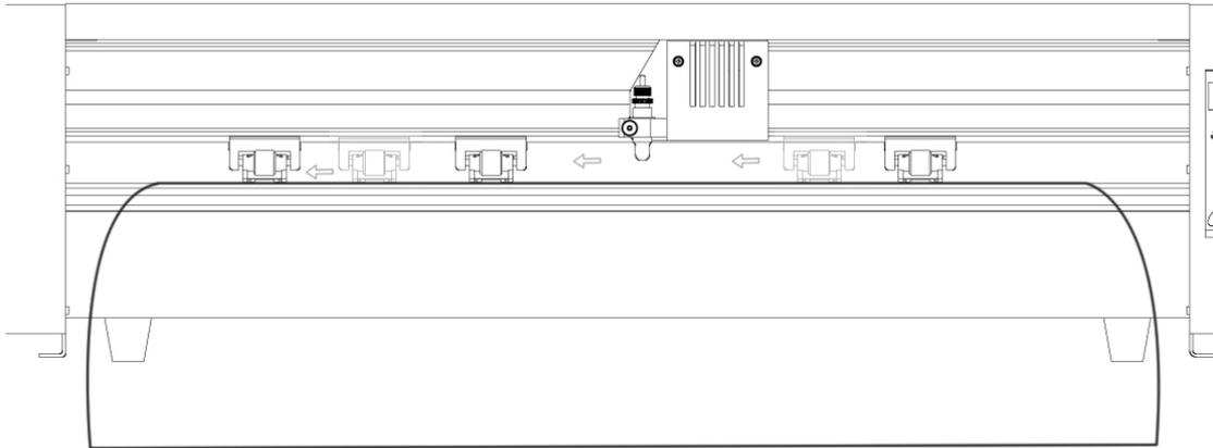
Leave a gap of between  $\frac{1}{2}$ "-1  $\frac{1}{2}$ " from the edge of the roller and the edge of the vinyl on both sides.
