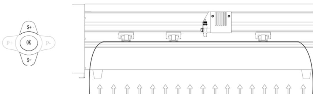
Adjust the carriage arm to the position where you want your cutting to start by using the Left and Right Arrow Keys.
