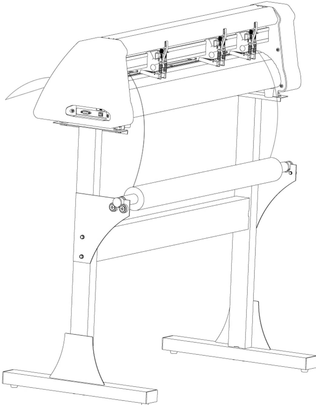
Adjust the pinch rollers so there is one roller located on each side of the vinyl (one cutter with 3 or more rollers, one roller near the center). Avoid lowering a pinch roller to the gap between the two feed rollers.
