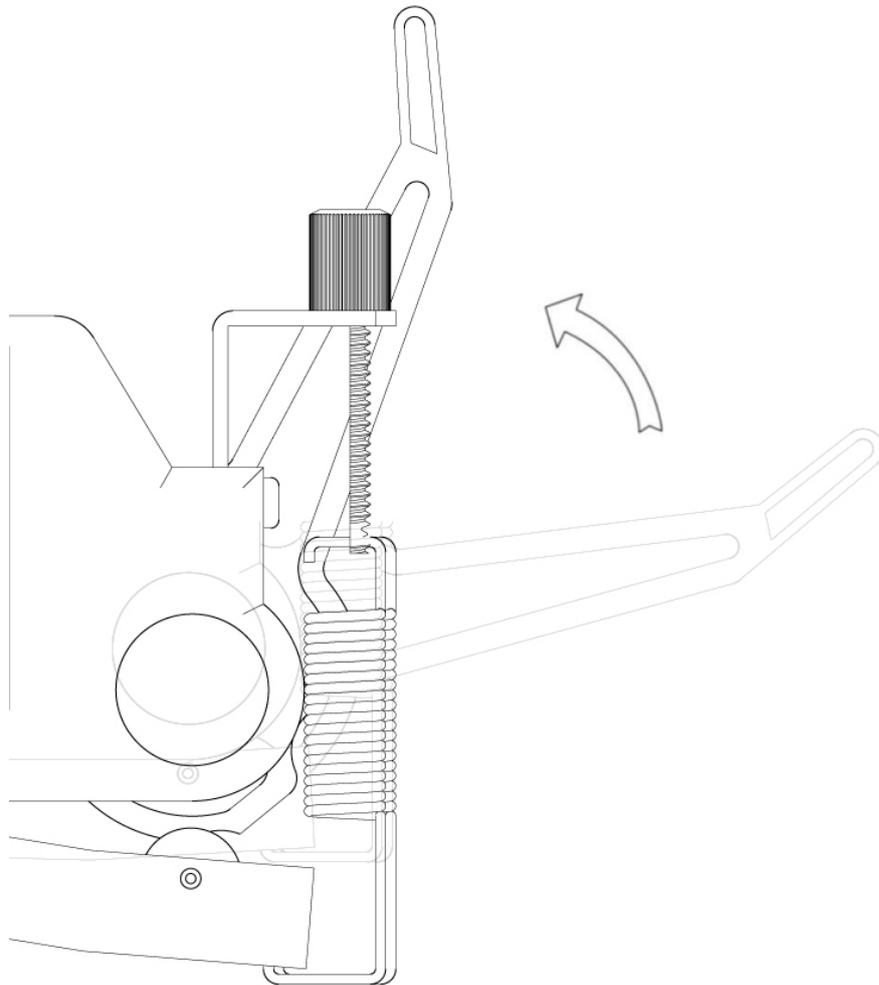
**Feed the vinyl underneath the pinch rollers (*if working from a single sheet instead of a roll, the vinyl can also be feed from the front*).**
