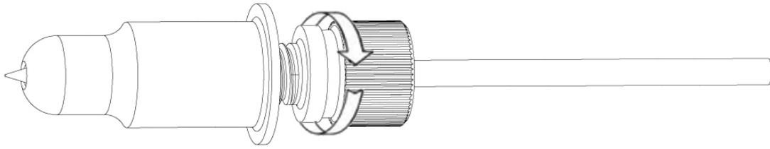
**Remove the top cap, the pen and the spring. Replace the pen and/or spring as necessary. Slide the spring onto the pen from the top and insert it back into the pen carriage.**
