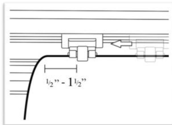
Engage the Pinch Rollers by pushing down on the Pinch Roller Release Levers.
